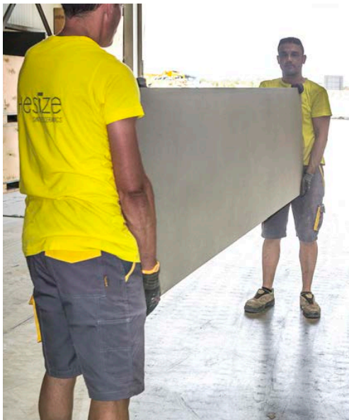
Image 8: Proper manual handling position
