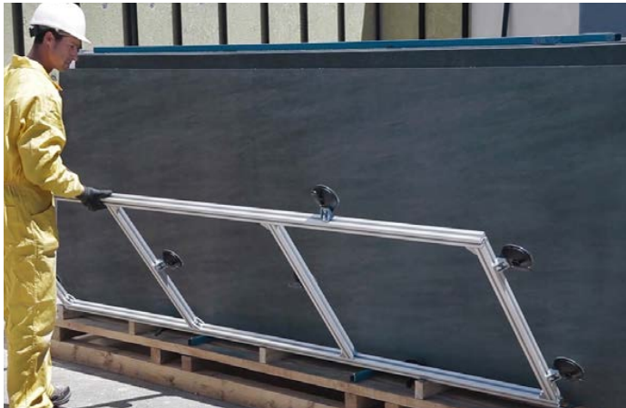
Image 6: Alimunium frame with suction cups
