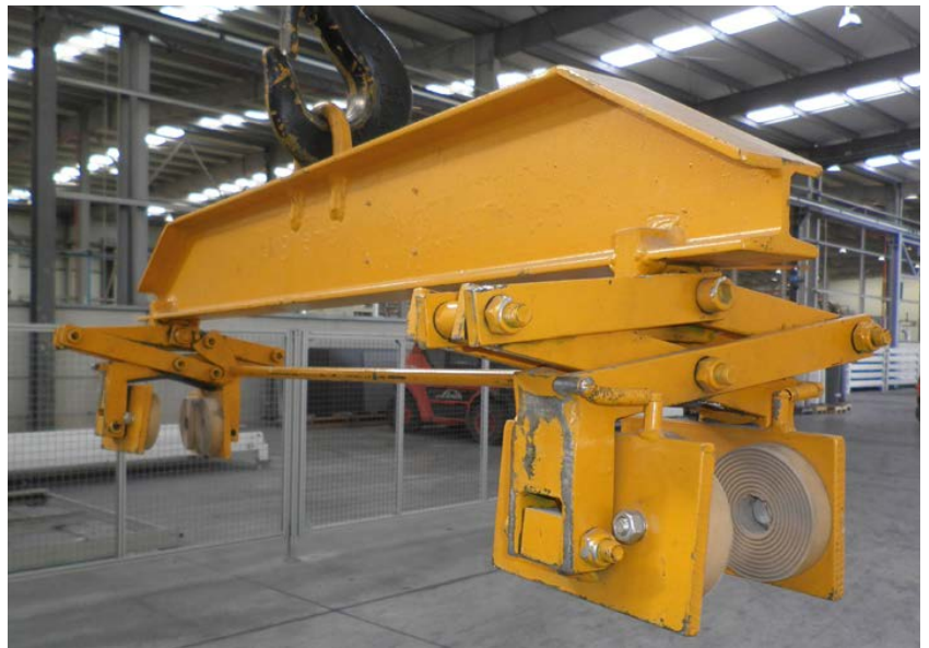
Image 9: Clamp handling for 12 mm slabs
